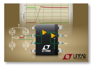
The LT1999 accurately measures fast switching currents in H-bridge motor controls, switching power supplies, solenoids and battery chargers. It features a –5V to 80V input common mode voltage range, 2MHz bandwidth, less than 1.5mV offset voltage and 0.5% gain error over temperature. With more than 80dB common mode rejection at 100kHz, the LT1999 maintains outstanding accuracy even in the presence of large square wave input voltages.
