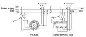
\* Grounding the secondary side of voltage transformer (VT) and current transformer (CT) is not necessary with low voltage circuit.
