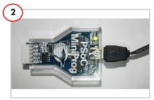
Remove the CY3217-MiniProg1 from the kit package; plug the USB cable into the USB Mini B connector and connect it to your PC.
