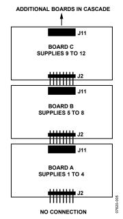
Figure 5. Connecting Multiple EVAL-ADM1186-1EBZs in Cascade
