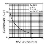
Fig.3 "ON" resistance vs. Input Voltage
