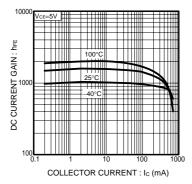
Fig.1 DC Current Gain vs. Collector Current
