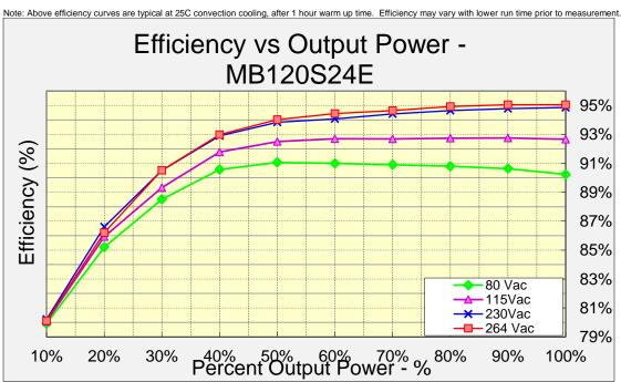
Note: Above efficiency curves are typical at 25C convection cooling, after 1 hour warm up time. Efficiency may vary with lower run time prior to measurement.
