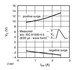
Fig. 6 - Typical Peak Clamping Voltage  $V_{\rm C}$  vs. Peak Pulse Current  $I_{\rm PP}$
