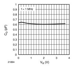
Fig. 3 - Typical Capacitance C<sub>D</sub> vs. Reverse Voltage V<sub>R</sub>
