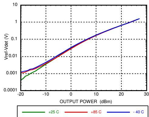
**Detector Voltage vs. Temperature @ 18 GHz**
